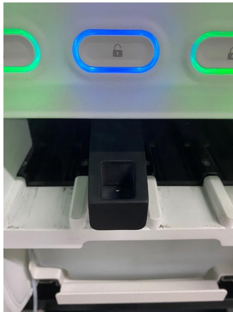
Figure 6-4 Properly install the reagent rack
