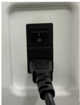
Figure 2-1 Power Cable Connection
