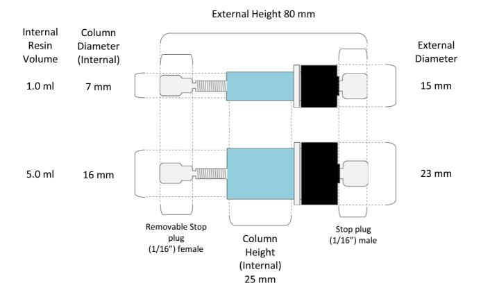
NOTE: HiFliQ FPLC columns are supplied with a moulded removable (1/16") female stop plug attached to the (1/16")
