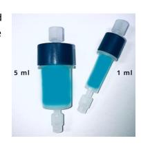
The Ni Advance Agarose resin provides high binding capacity with minimal Ni<sup>2+</sup> ion leakage for high stability, chemical compatibility and reuse. Compatible with all common liquid chromatography instruments (including ÄKTA™ FPLC's), peristaltic pumps and syringes.
